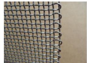
**Raw edge** is where there is no retaining loop of the Weft wire around the outer edge of the weave. This typically occurs in meshes where the crimp is sufficient of itself to prevent unraveling and also in intermediate crimp specifications.
