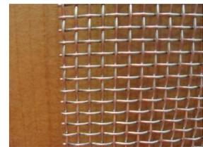
**Mixed edges** are when the weave has a Selvedge and raw edge. This will occur when the mesh is woven with a Selvedge edge and then the width is cut down.
