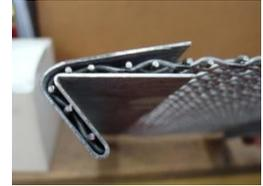
**Selvedge edge** is where the Weft wire loops around the outer Warp wire prior to returning across the weave, providing finished edges, which prevent unraveling.
