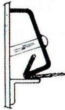
7. Engage clamping bars securely into hooked edges taking care they clear any sheetmetal lip.
