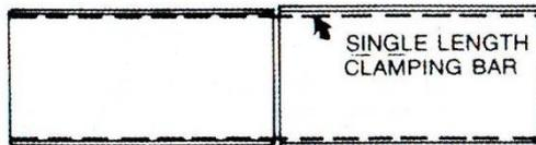
We DO NOT recommend the tensioning of two or more screencloths with a single clamping bar, as there can be variation in screencloth width, which results in the wider cloth not being held in correct tension.
