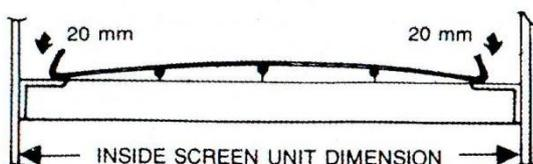
Generally the overall hooked edge dimension is the inside dimension of the unit less 40mm. This provides for 20mm clearance to each side of the screencloth.
