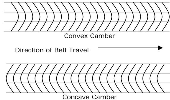
Camber in a high temperature belt may be either convex or concave as shown above, or, in some cases, the camber may develop with one edge of the belt leading the other edge.
