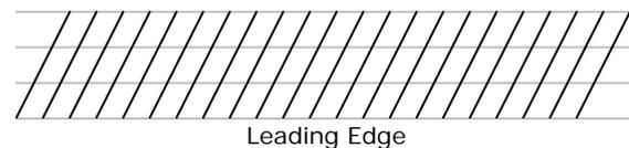
It is frequently caused by such factors as uneven loading, uneven temperature, drafts in the cooling chamber, uneven driving tension, or a combination of these factors.
