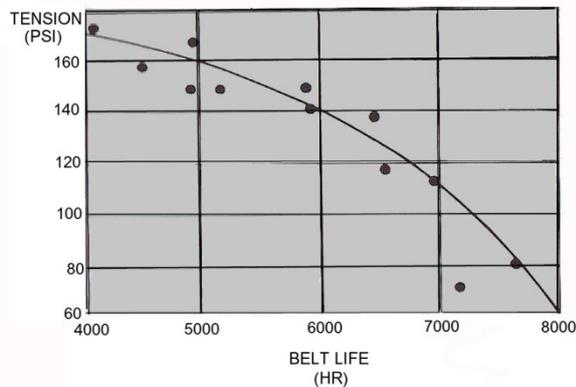
This study was primarily concerned with copper brazing belts operating at 1121°C, but the results are generally applicable to all types of high temperature belts. Every effort should be made to maintain operating tension at the lowest possible value.
